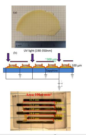
**FIG. 1.** (a) Optical image of a portion of the diced h-<sup>10</sup>BN sample used in this work. (b) Schematic diagram of detector strips mounted on a sapphire sub-mount with UV light illuminated through a metal mask, allowing the measurement of electron and hole transport separately. (c) Optical image of a 1 cm<sup>2</sup> neutron detector fabricated from a 100  $\mu$ m thick h-<sup>10</sup>BN freestanding wafer by combining five detector strips.
