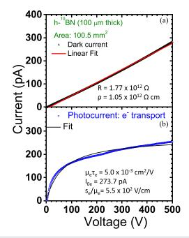
FIG. 2. Current–voltage characteristics measured for the device configuration shown in Fig. 1(b): (a) in the dark and (b) under UV radiation for electron transport.
