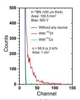
**FIG. 3.** Pulse height spectra of the 1 cm<sup>2</sup> h-<sup>10</sup>BN detector. The red curve is the response to thermal neutrons which was recorded by placing the detector 1 m away from the <sup>252</sup>Cf source moderated by a HDPE cube. The blue curve is the background (or dark) counts measured at the same bias voltage. The green curve is the response to gamma photons emitted from a <sup>137</sup>Cs source measured at the same bias voltage.
