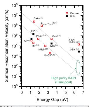
FIG. 4. Surface recombination velocities of representative semiconductors vs the energy bandgap  $E_g$ , with published data from Ref. 23 for GaAs, Ref. 18 for InP, Ref. 24 for Al<sub>0.51</sub>In<sub>0.49</sub>P, Ref. 20 for InGaN, Ref. 19 for InGaP, Refs. 21 and 22 for GaN, Ref. 25 for Si, Ref. 26 for 4H-SiC, and Ref. 16 for h-BN. The black lines serve as a guide to the eye revealing the trend of decreasing surface velocity with an increase in the energy bandgap of semiconductors.
